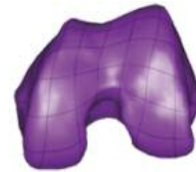
Figure 1. The unique shape of each patient's bone is modeled from a CT scan and the implant is manufactured to match the shape and size.
